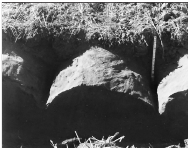
Figure 6.23 Ripper shanks spaced 30 inches apart produce channels without any overlap and therefore leave much compacted soil unloosened. Depth of ripping is 16 inches.
