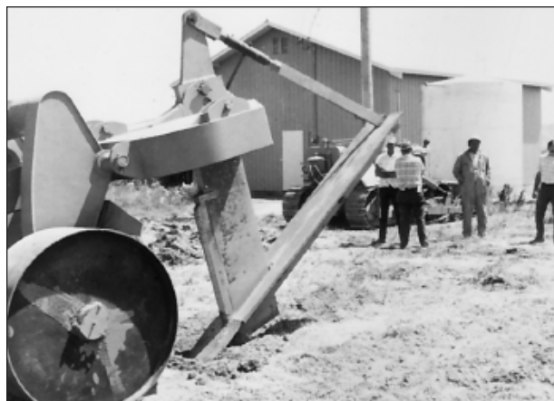
Figure 6.18 With the shank shown, this slip plow can operate almost 5 feet deep. The slip plate is 15 inches wide.
