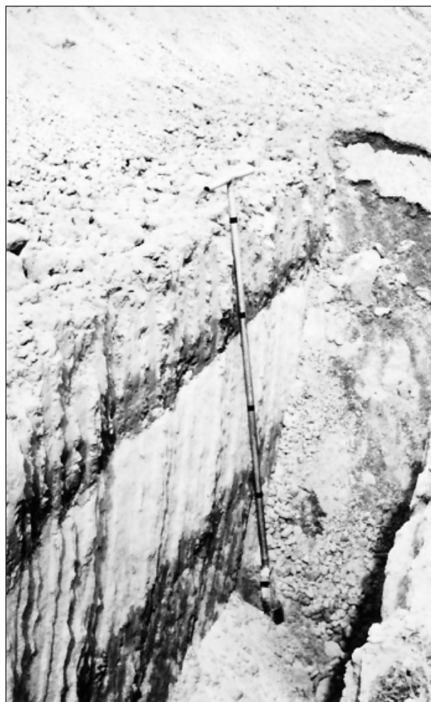
Figure 6.3 This stratified floodplain soil with an abrupt interface boundary between a fine sandy loam surface soil and white sand subsoil that limits root development and water movement. Note the wet zone immediately above the sand layer.
