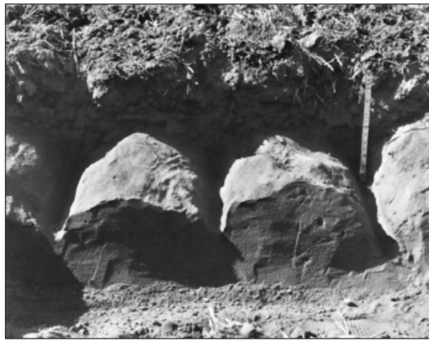
Figure 6.24 When shank spacing is reduced to 20 inches, much more soil is loosened. Normally, the lower one-third of the shank makes almost straight-walled channels which fan out toward the less confined soil surface.
