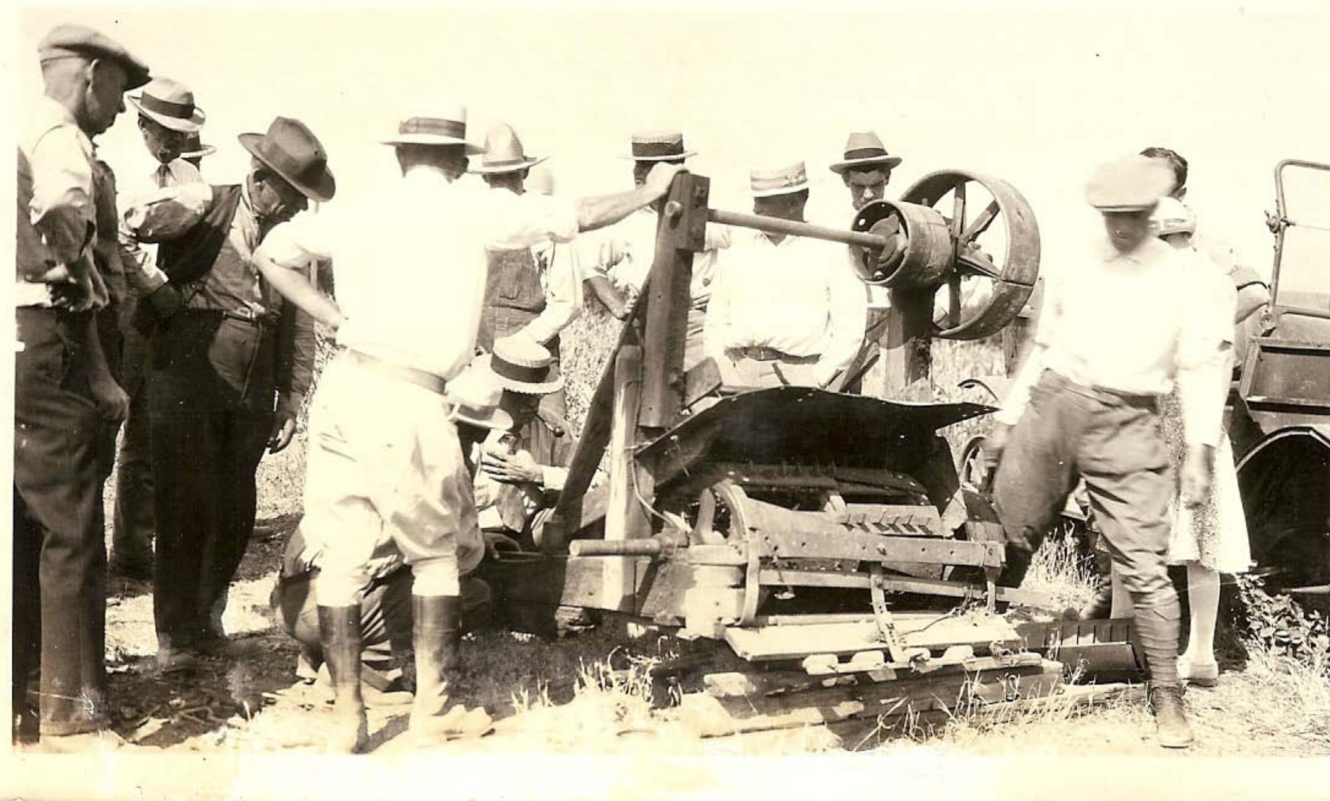
Growers checking the cylinder type of shredding machine by Noble at Orosi. Source: Alan George
