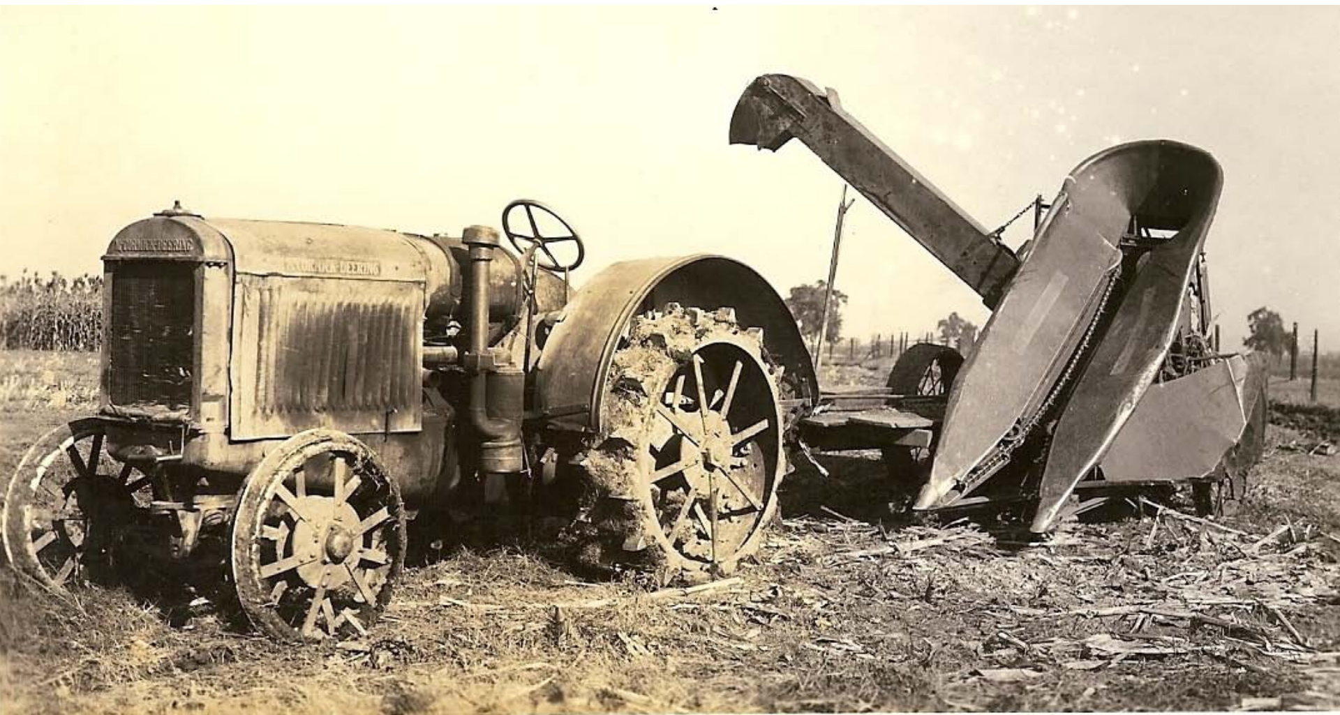
Field corn or sorghum harvester. Mc Deering track layer tractor. Source: Alan George, Norm Phillips and Wayne Collins.
