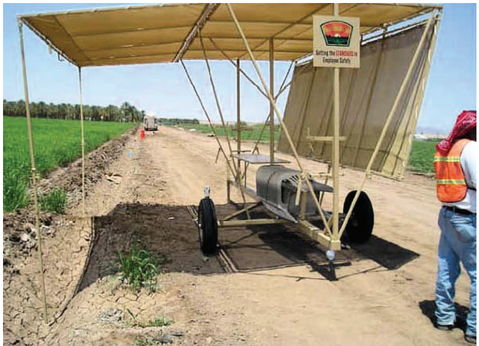
Figure 2. Mobile pop-up shade units allow workers to work or break in an area protected from direct sunlight.
