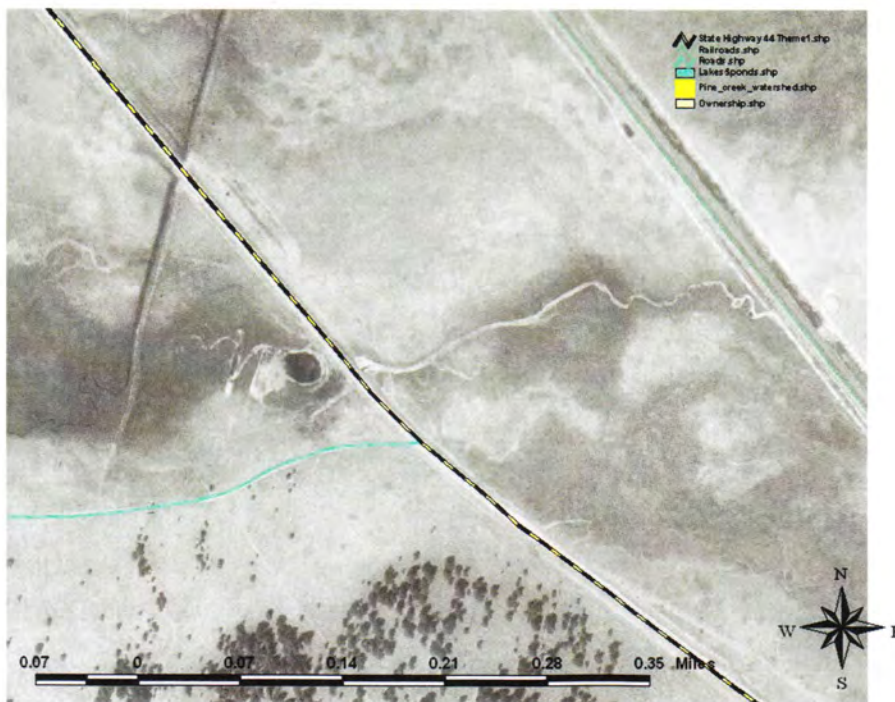
Figure 19a. Aerial images of, at top: reconstructed channel showing newly constructed berms downstream (see arrow), culvert at railroad grade, and berm removal upstream of the pond on Pine Creek, and bottom: channel as it existed from the 1950's through 1999, carrying only flood flow and draining alongside railroad line.
