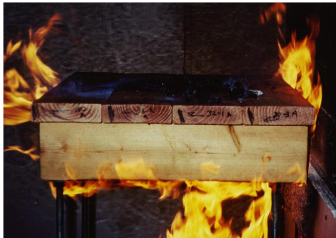
Figure 7. When deck boards are butted, flames cannot easily penetrate between board spaces. The rate of thermal degradation of the deck is minimized.
