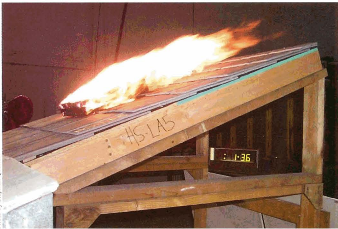
At the beginning of the fire test, a burning "A" brand is placed on top of the roof deck. The test continues until the brand and material in the deck stops burning, or until flame penetrates through to the underside of the deck.
