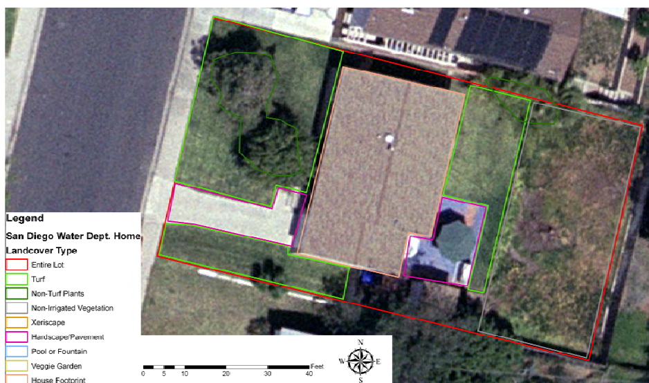
Figure 22: Example of using digital imagery and geographical information system tools to calculate landscape area
