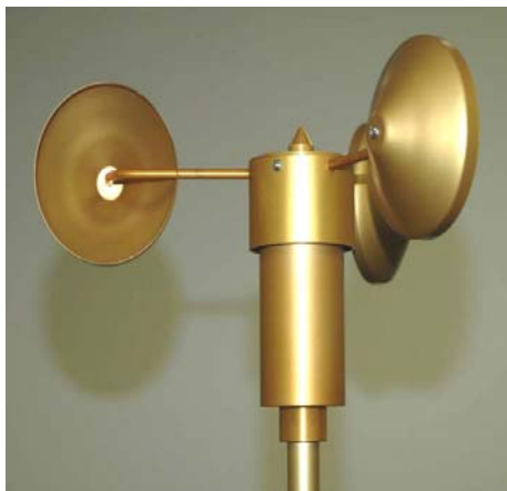
Figure A 19: Calsense anemometer
