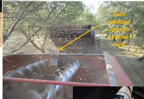
Hydraulically driven auger to deliver samples to rear
