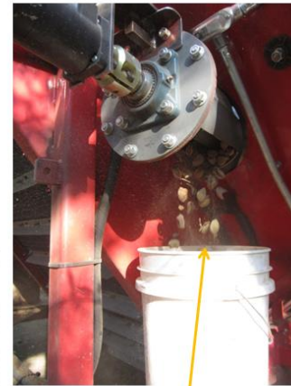
Samples are delivered to 5 gallon bucket at rear (much safer than old method of getting samples by hand)
