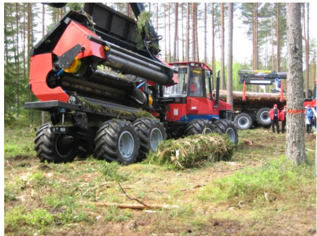
Biomass bundler on a Valmet 860 forwarder frame; shown at an equipment demonstration believed to be in Elmira, Oregon. June 2005. Photographer unknown
