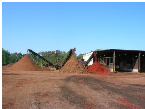
The Scotts Company, Naturescapes mulching operation, Waverly, Virginia. Mulch is chipped and colored before bagging or bulk sale. May 18, 2006. John Stewart
