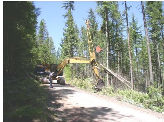
An "excaliner" yarder is capable of yarding biomass from small diameter timber stands growing on steep ground. It can also operate off-road to some degree. Bonners Ferry Idaho, June 2004. Photo by Barry Wynsma, USFS
