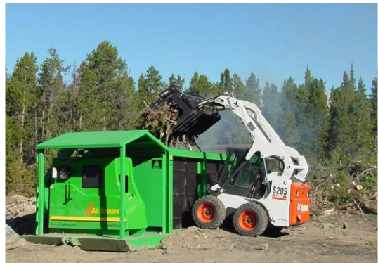
Meeker Park Collection Site/Sort yard showing the loading of Boulder County's Air Curtain Burner, Date: Summer 2008. Photo by Craig Jones, CSFS Project Manager for Peak to Peak Wood.
