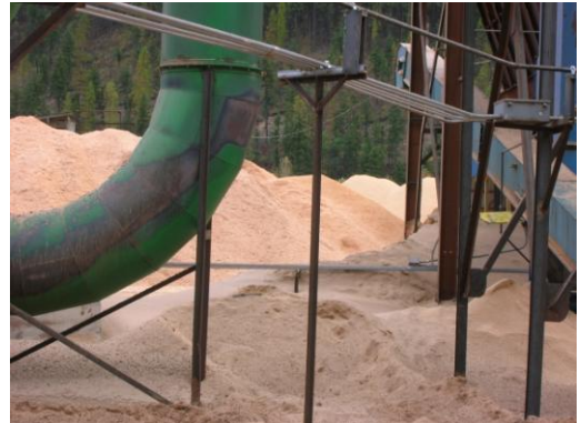
Potential fire threat from fine dust particles at the Eureka pellet in Superior, Montana. October 12, 2005. John Stewart
