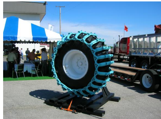
High flotation tire for low ground pressure skidder; photo taken at SmallWood 2006 Conference in Richmond, Virginia. May 19, 2006. John Stewart
