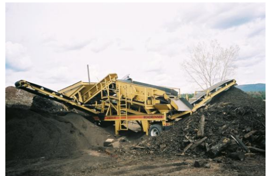
Screen sorting log yard debris, Fort Apache Timber Company, Whiteriver, AZ. Source: USDA Forest Service
