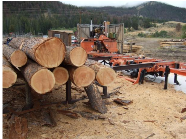
Thin-kerf band sawmill operation. Dubois, WY. Source: USDA Forest Service
