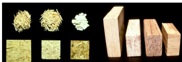
Wood composites from woody biomass furnish. Forest Products Laboratory, Madison, WI. Source: USDA Forest Service
