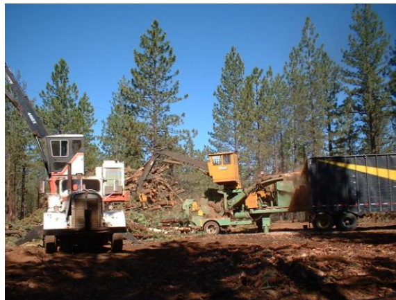
Chip truck loading in a hot landing, Eagle Lake Ranger District, Lassen National Forest. July 18, 2003. John Stewart
