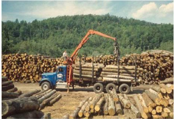
Log truck with hydraulic self-loader. Source: USDA Forest Service
