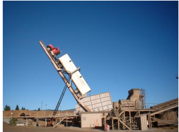
Chip truck off-loading via hydraulic lift at the Mt. Lassen Power plant, Westwood, California. September 18, 2002. John Stewart
