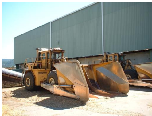
Large scoop for moving and loading wood chips at Burney Mountain Power, Burney, California. July 17, 2003. John Stewart
