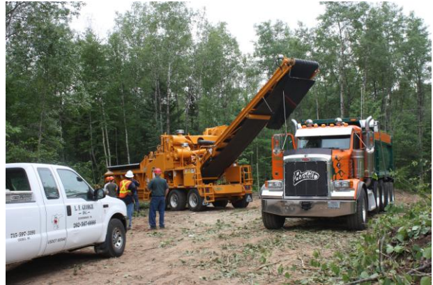
In-woods biomass grinder loading energy chips. Source: USDA Forest Service
