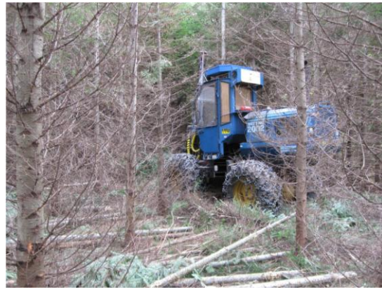
Rottne 2002 “mini-harvester”. This machine is less than 8 feet wide and can reach about 23 feet with the harvester head. The machine is shown operating in an overgrown grand-fir Christmas tree plantation in Bonners Ferry, Idaho on private lands in 2008. Photo by Barry Wynsma, USFS October 2008
