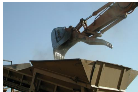
Loading urban wood waste into a screen hopper; Carson City, NV. Source: USDA Forest Service
