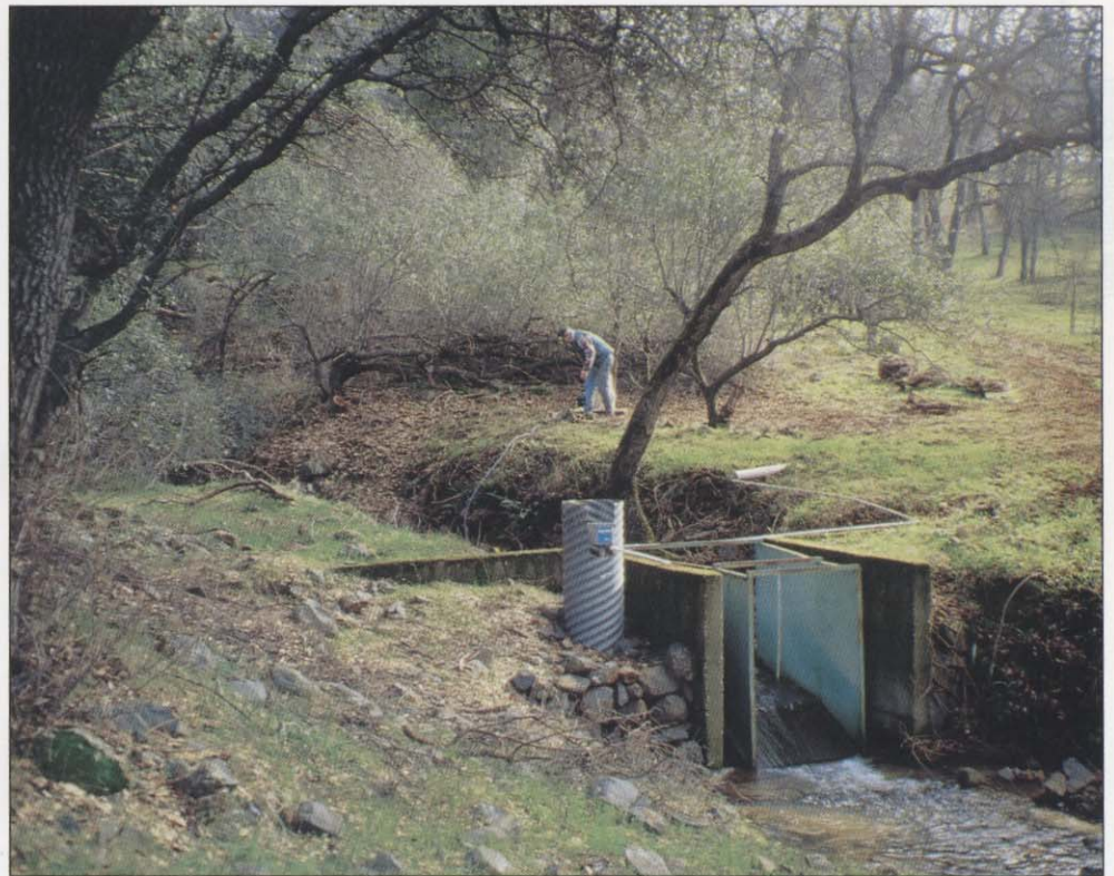
Stream flow is measured and recorded every 15 minutes.
