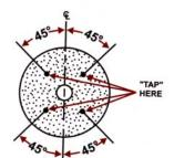
Suspend wheel from the hole by a metal pin or finger
