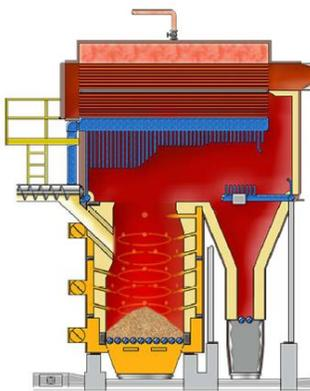
Figure 4-6 Wellons Biomass Package Boiler
