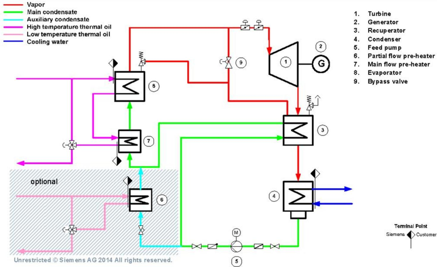
Figure 2-6 Typical Easily Modularized ORC Equipment
