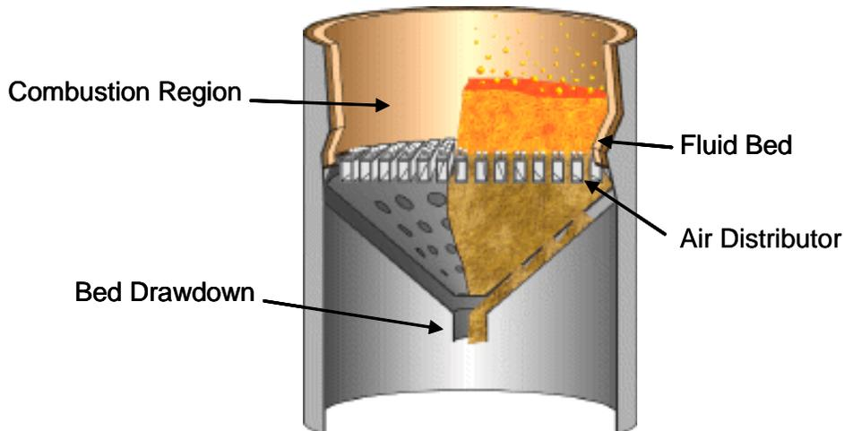
Figure 2-2 Typical Bubbling Fluidized Bed (Source: Outotec)
