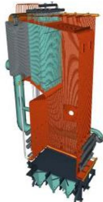
Figure 4-2 FSE Energy Traditional Stoker Boiler
