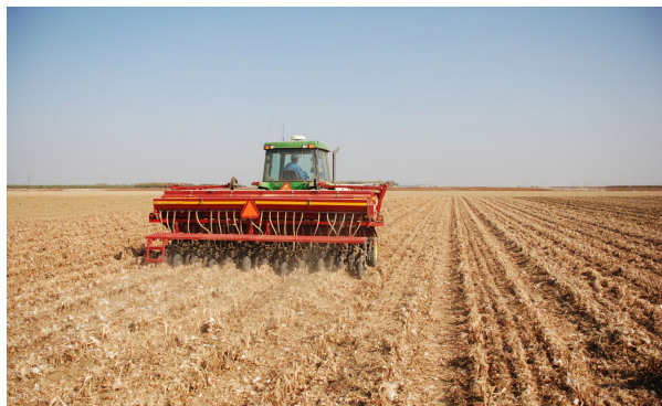
Figure 2. Cover crop seeding using Sunflower 3-m no-tillage grain drill into cotton, tomato and previous cover crop residue in Five Points, CA
