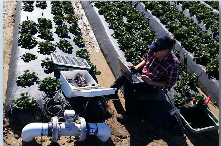
Staff Research Associate Kamille Garcia downloads flow meter data of irrigation scheduling study.
