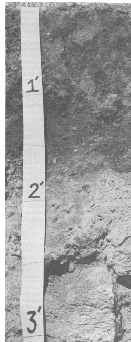
Figure 4.—Profile of Exeter sandy loam, 0 to 2 percent slopes. A duripan is at a depth of about 24 inches.
