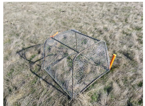
Cages such as the one pictured here are one way to exclude grazing from small areas. We can then measure total forage production at the peak of the growing season.
