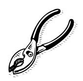
Pliers are hand tools with two handles that function as levers about a pivot hinge. Most types of pliers have serrated jaws located at the tips. Pliers are primarily used for gripping, twisting, turning, and cutting objects. Common types of pliers include adjustable or slip-joint pliers, needle-nose pliers, channel-lock pliers, lineman's pliers, vise grips, and diagonal- or side-cutting pliers.
