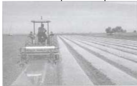
Figure 2. Applying polyethylene tarps on 42-inch (105-cm) beds with a mechanical tarp layer.
