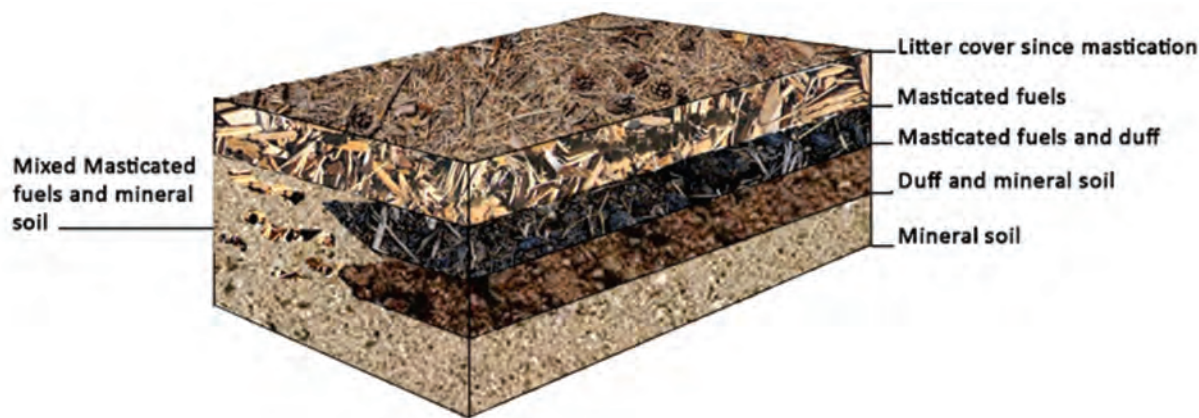
Figure B.2 —A cross section of the masticated fuelbed illustrating the five fuelbed layers that were characterized in this study.
