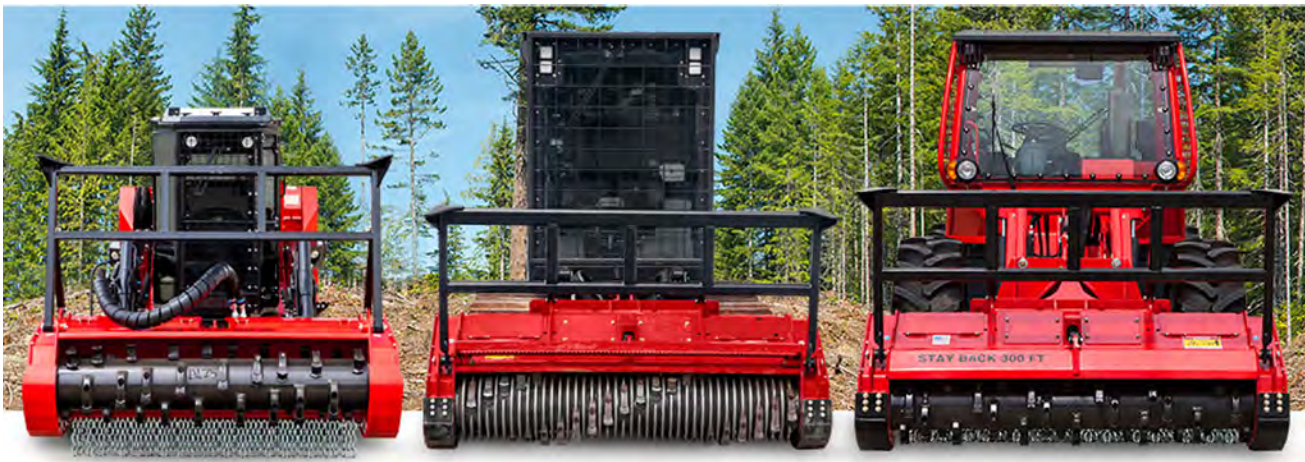
Figure 4 —Horizontal shaft cutting heads can have knives or teeth designed to work in different settings, such as on rocky soils (photographs provided by Fecon Inc.).
