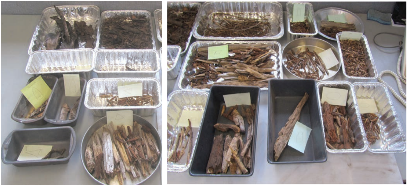
Figure 6 —Masticated fuel particles from one sample bag, sorted by shape (table 5) and size: (a) masticated fuel shapes and (b) other fuel shapes.
