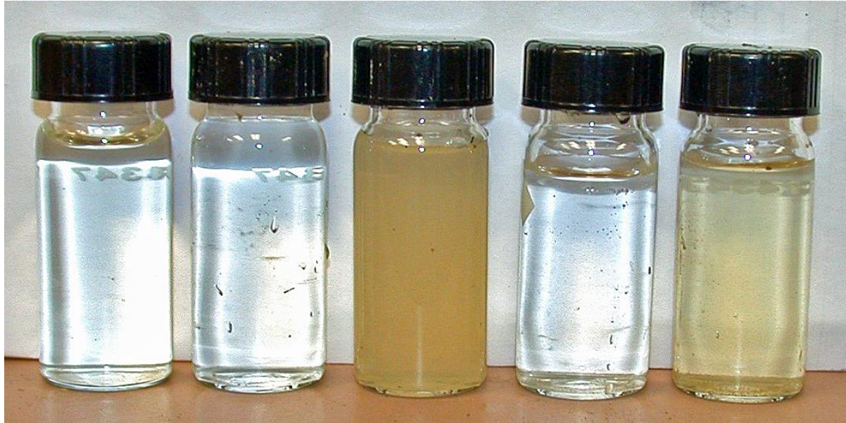
From left to right: Turbidity of runoff from post rows with: mulch, weed barrier fabric, bare soil, polyacrylamide and barley cover crop
