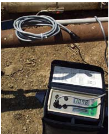
Figure 3. Ultrasonic (Doppler) flowmeter. Photo: Lawrence J. Schwankl.
