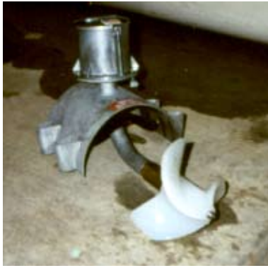
Figure 1. Propeller flowmeter. Photo: Lawrence J. Schwankl.
