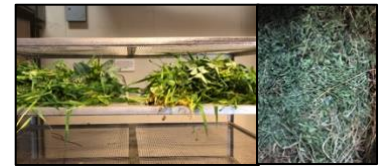
Images 12-13. Biomass drying in an oven (left). Dried material after 48h (right).
