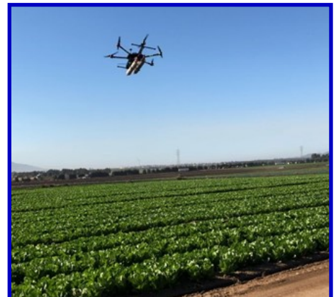
Drone releasing beneficial insect predators of aphids on organic Romaine lettuce near Soledad, CA.
