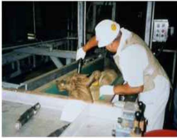
Captive bolt stunning in center track restrainer
