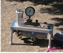
Soil Moisture Equipment Plant Pressure Chamber
