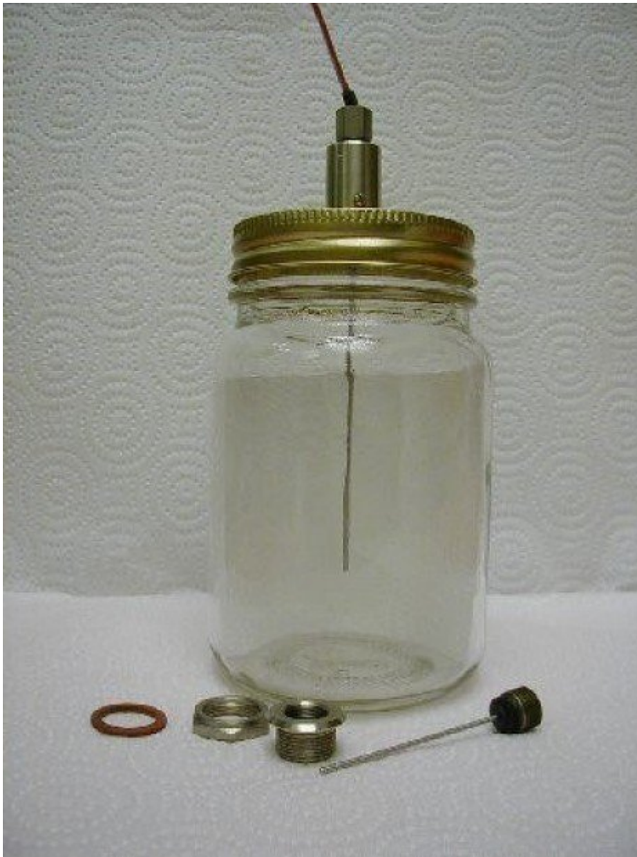
Thermocouple for testing temperature inside jar: National Center for Home Food Preservation
