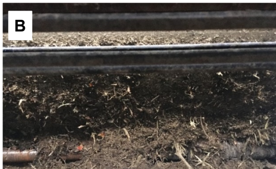
Figure 5. A tomato harvester (A) and soil and plant debris buildup on parts (B). Photos taken by Cassandra Swett.
