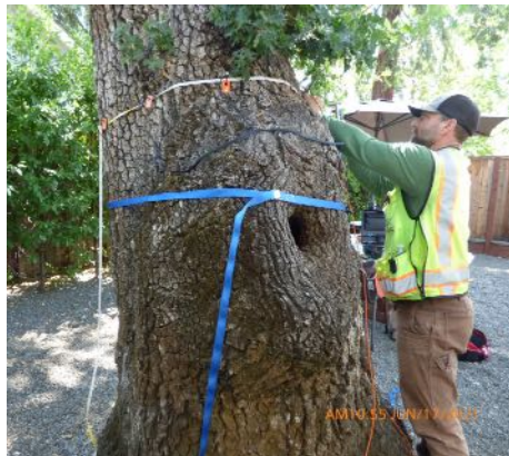
An arborist using a tomograph, a tool used to detect decay and assess the interior health of a tree. Photo by Denise Britton.
