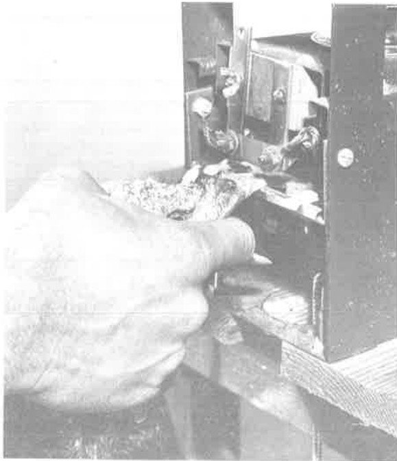
Fig. 8. Cannibalism can be avoided by using an electric de-beaker.
