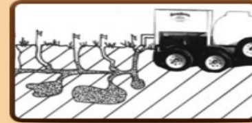
Diagram of how the Burrow Blocker effectively fills ground squirrel holes and burrows.
