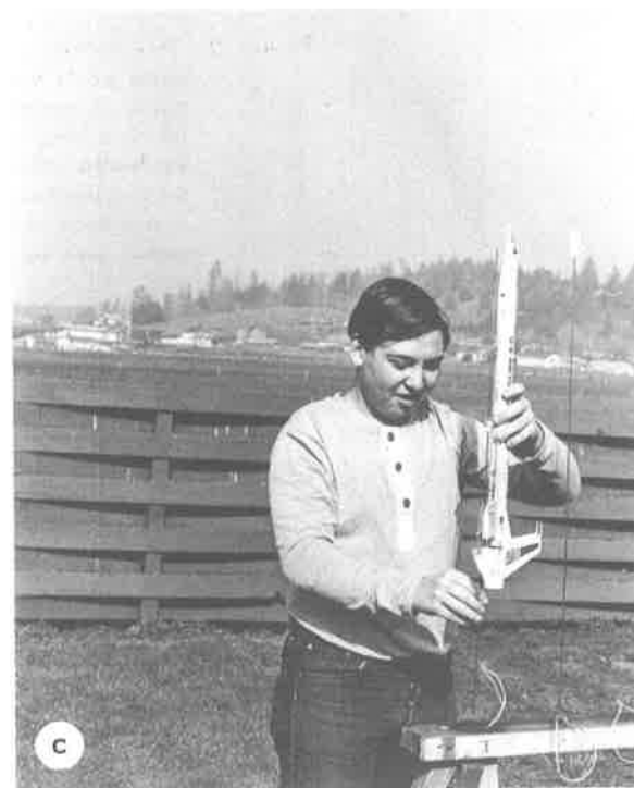
Figure 19. a) In assembling the rocket launch pad, make sure that launch rods are straight and that they make a good connection with the launcher circuitry. b) Then place the rocket on the launching rod. c) Take care not to break the rocket or the launching-rod lug and make sure you do not disrupt the launching-rod circuit.
