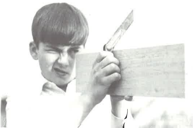
Chamfers, as illustrated above, and bevels may be tested with a T bevel.
