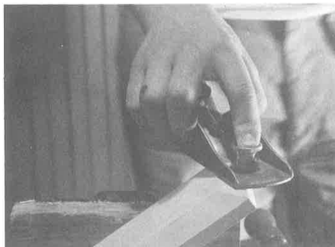
The block plane works well to cut chamfers and bevels.
