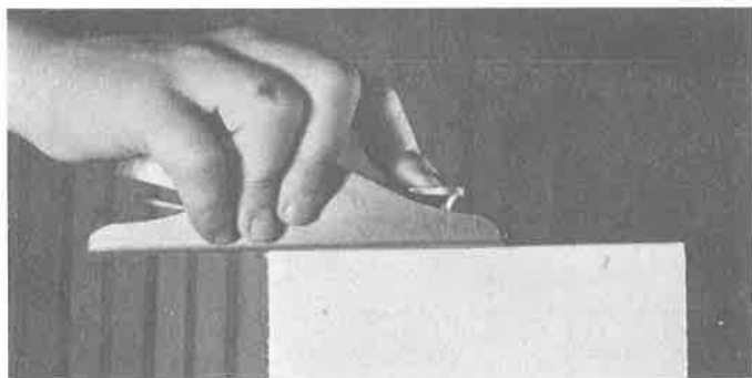
Because of the low angle, the block plane is used for fine work and end grain.
