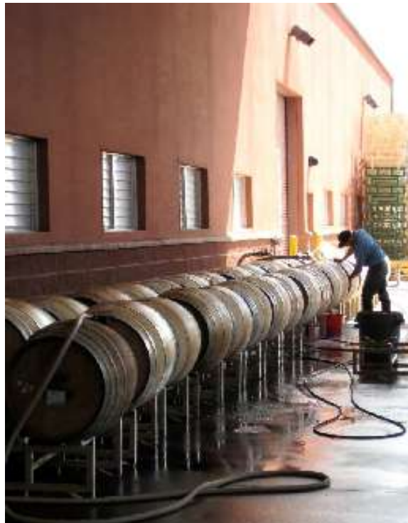
Installing timers for barrel washing, along with using a high pressure/low volume nozzle, helps conserve water needed for barrel sanitation.
