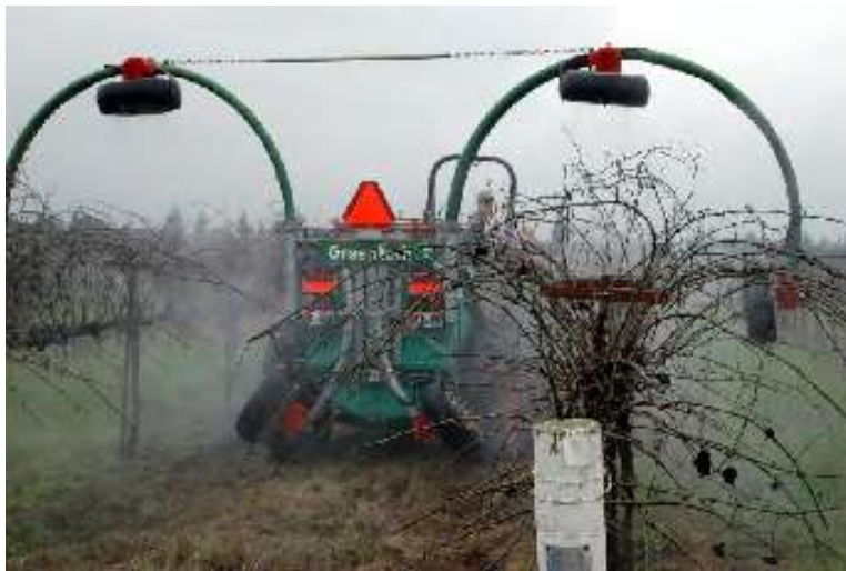
Low-drift spray technology can help reduce drift by pesticides.
