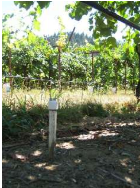
Soil moisture monitoring devices are used to accurately schedule irrigation for efficient water use.
