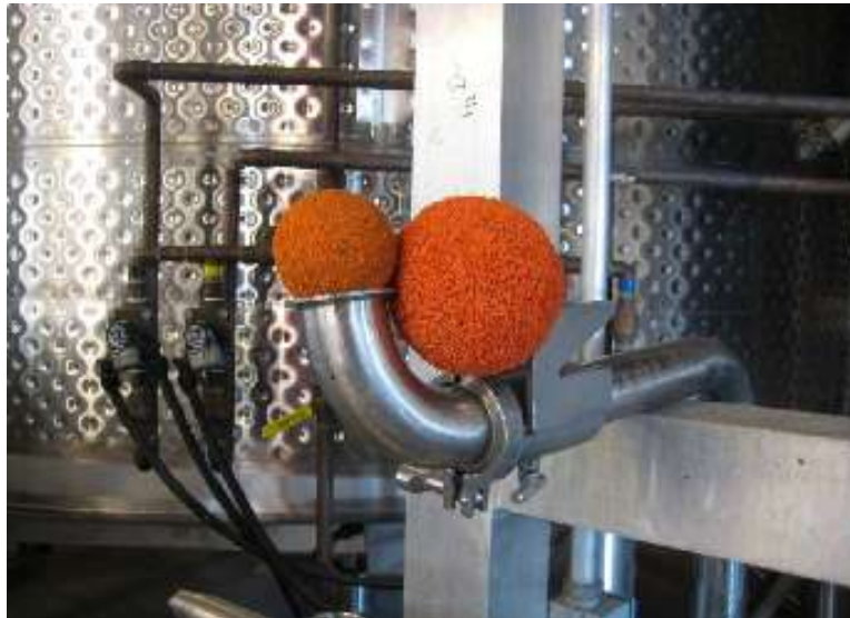
“Pigging” is a common sanitation option that can save a lot of water when cleaning transfer lines.
