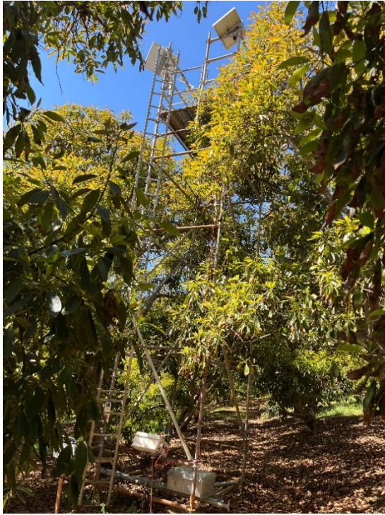
Fig. 2. Ground view of a flux tower/monitoring station in an avocado orchard in Irvine.
