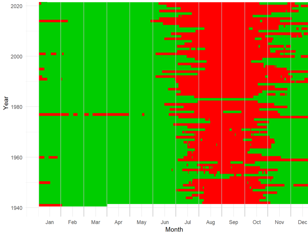
Figure 25: Heat map that is indicating, in red, days (x-axis) of each calendar year (y-axis) during which historical flows measured at the USGS Fort Jones gage on the Scott River were less than 100 cfs.
