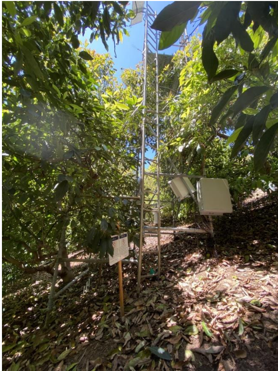
Fig. 4. Ground view of surface renewal and eddy covariance ET station at the avocado site in Escondido.
