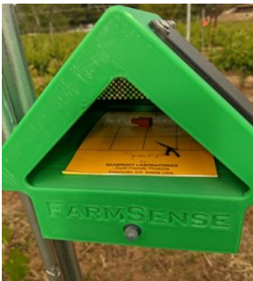
Insect trap with wireless optic sensor
