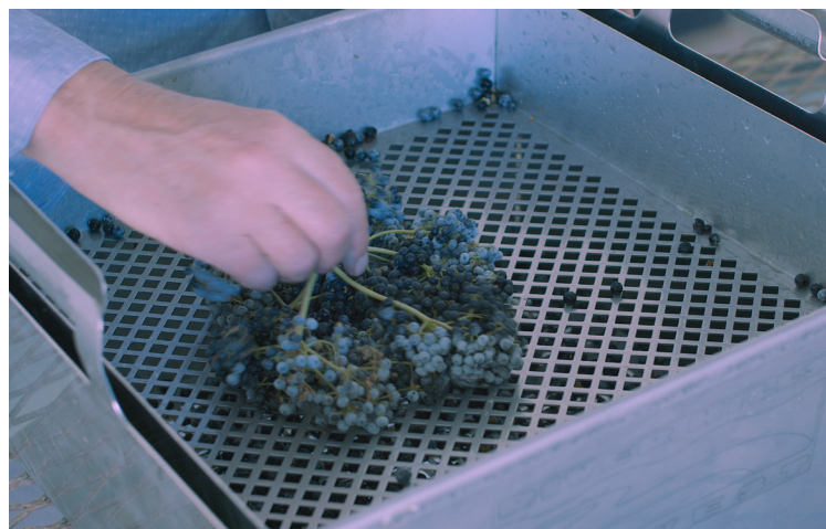
Figure 7. A stainless steel elderberry destemmer can assist with removing elderberries from stems through gentle rubbing across the screen to release elderberries through the holes. Photo by Ethan Ireland.
