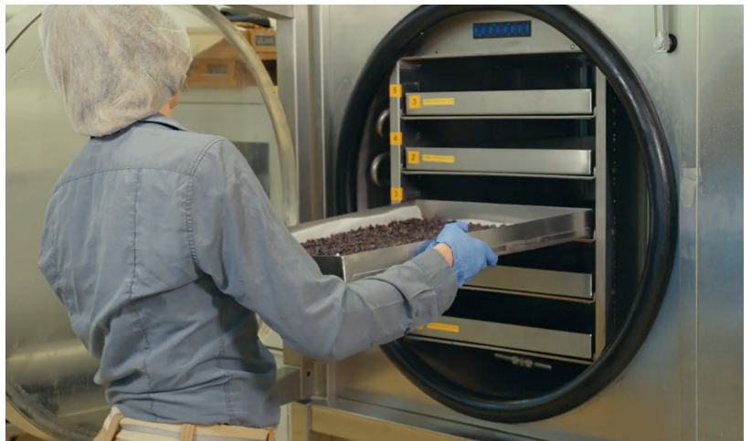
Figure 3. Freeze dryer, which can be used to dehydrate elderberries. Operational, equipment, and energy costs for freeze drying are much higher than those for other drying systems. Photo by Ethan Ireland.
