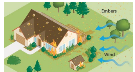
Figure 1 (Top) Movement of fire through contiguous vegetation (Bottom) Ignition of near-home landscaping from embers (Valachovic et al, 2021).
