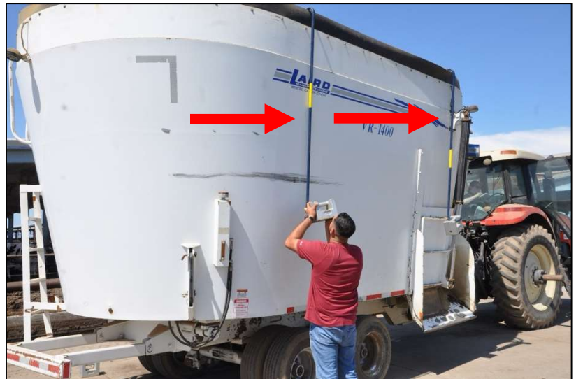
Picture: UC Davis student adding 50-pound standard weights to each individual bar after placing the four pipe hooks. Red arrows identify the pipe-hooks.
