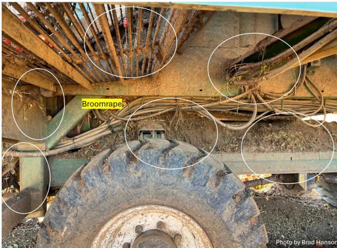
Tomato harvester undercarriage, following the harvest of a broomrape-infested field in Chile.
